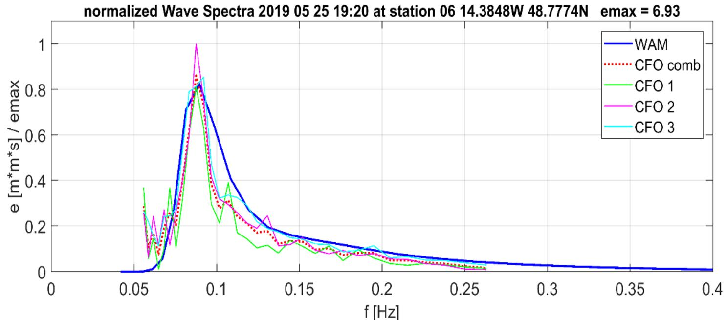
*Filtered 1D-Spectra. Spikes in the low frequency range of the combined spectrum (red dotted line) are also visible in the 6° beam spectrum (CFO 1, green line).*
