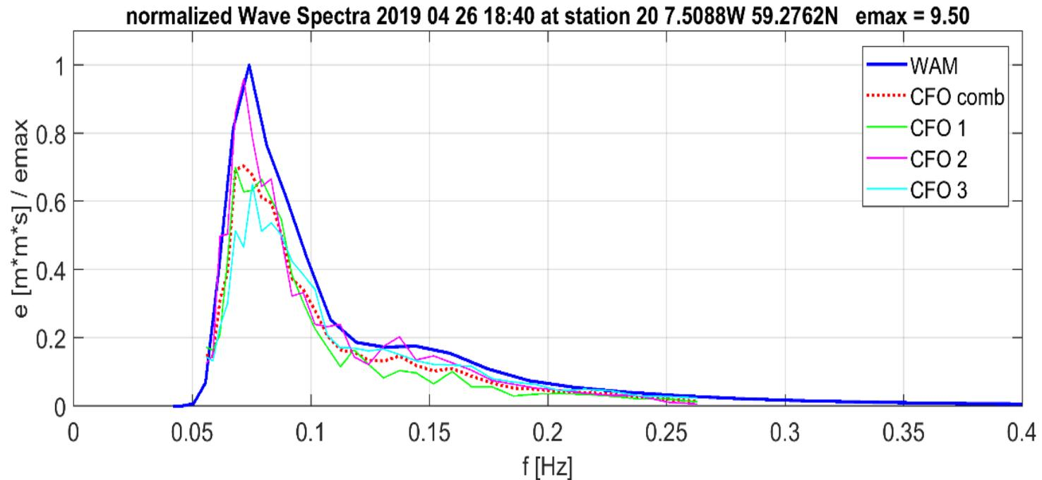
*Filtered 1D-Spectra. Spikes in the low frequency range of the combined spectrum (red dotted line) are also visible in the 6° beam spectrum (CFO 1, green line).*
