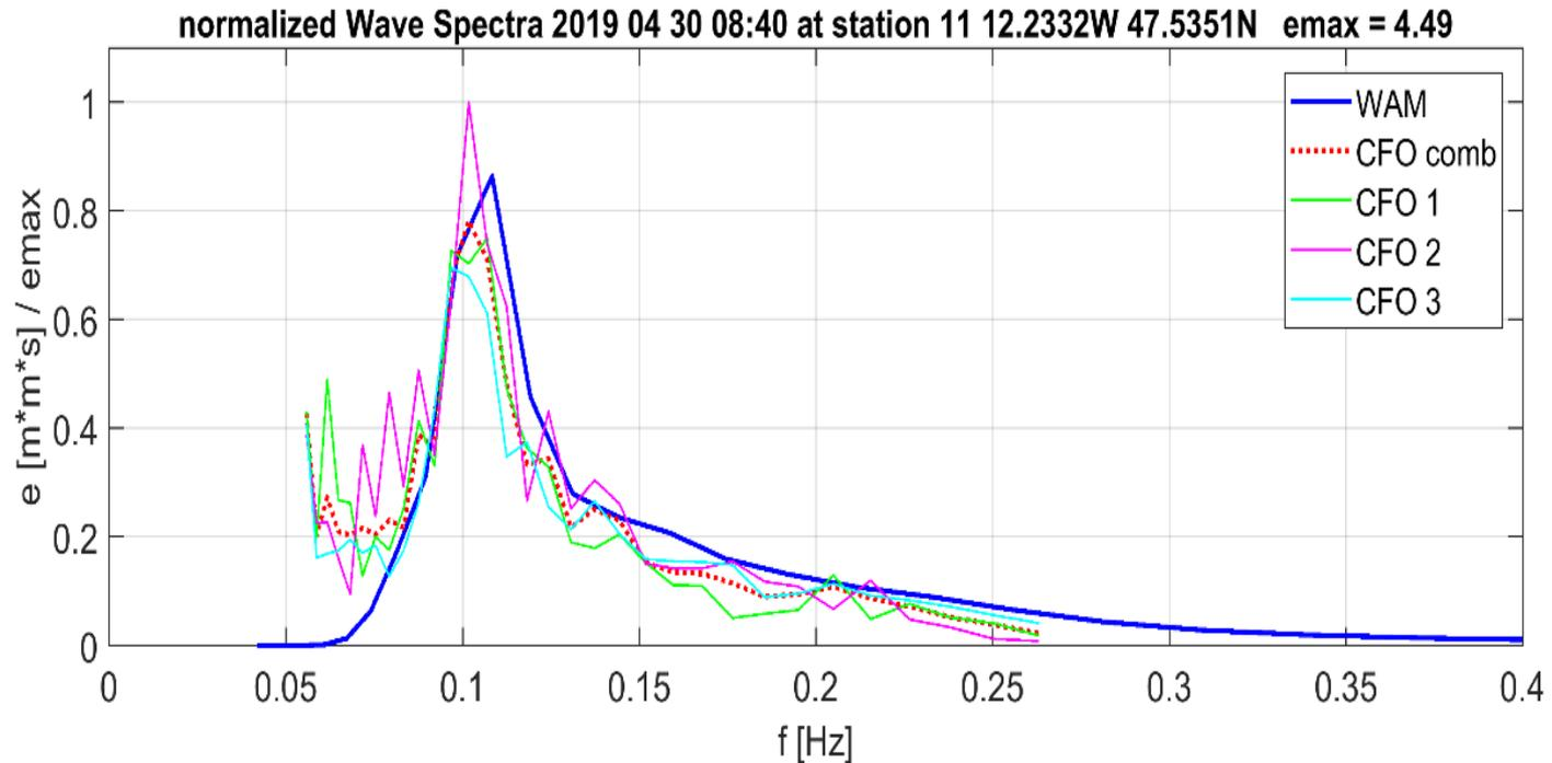
*Filtered 1D-Spectra. Spikes in the low frequency range of the combined spectrum (red dotted line) are also visible in the  $6^\circ$  beam spectrum (CFO 1, green line).*
