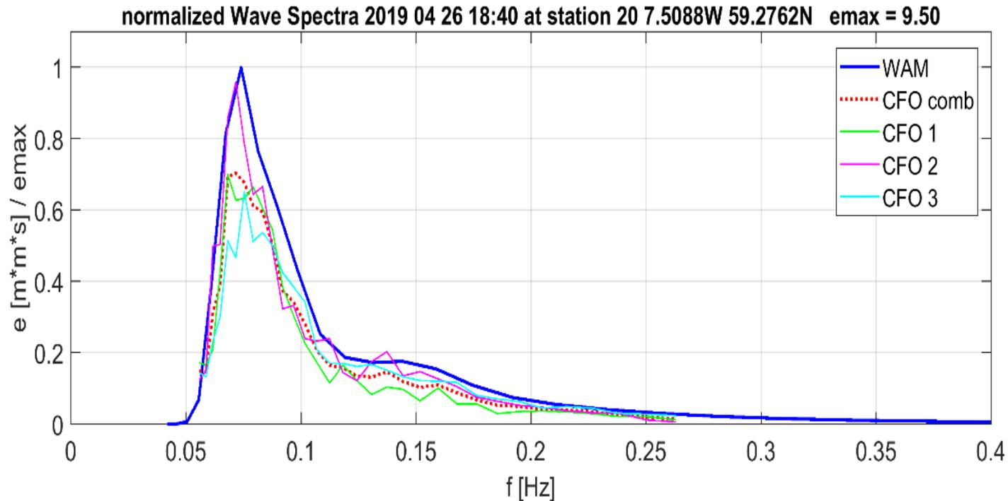
Filtered 1D-Spectra. Moderate damping of the combined CFOSAT spectrum, stronger at lowest frequency. Reduced peakedness.
