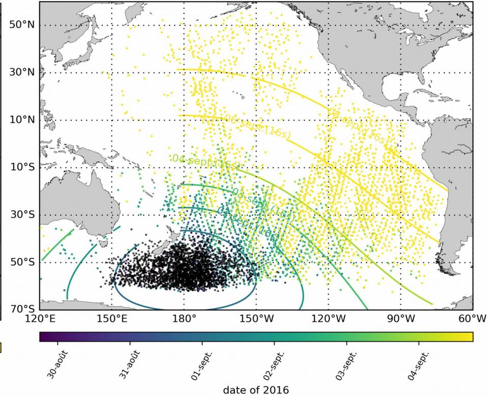
Example of wave observations (colored dots) associated to a storm source. Back-propagated observations are black dots.
