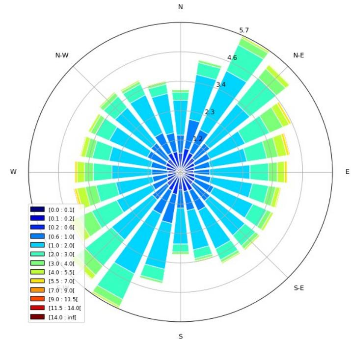
Example of joint distribution,  $H_s$  and wave direction (wave rose)
